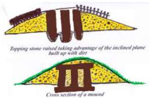
Fig. 2 The capping megalith raised by pulling along an inclined plane and covered as a mound
